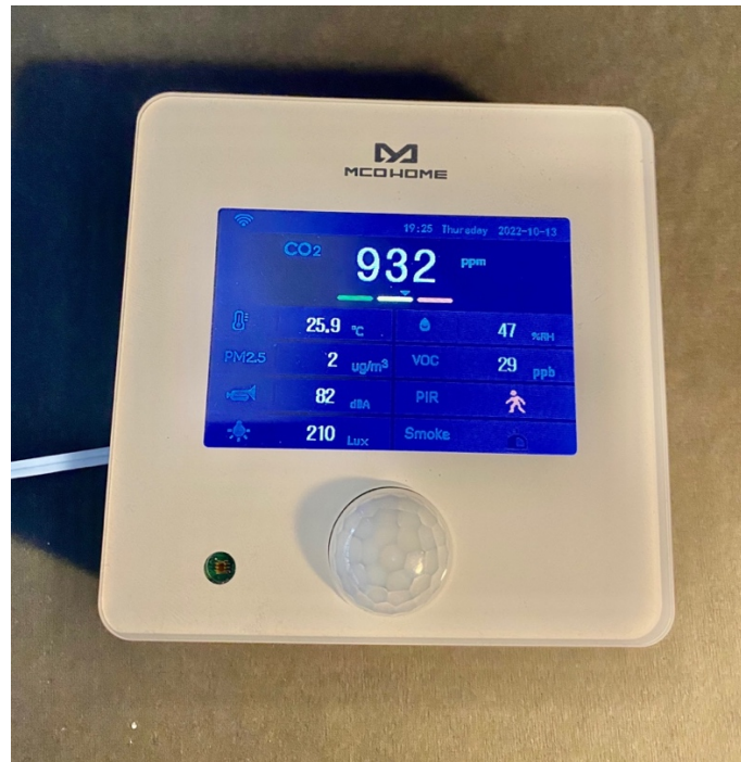
Figure 9. Second tested case for Indoor Air Quality multi-sensor
