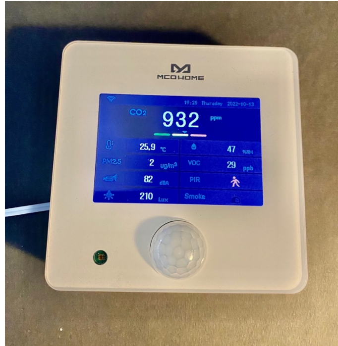
Figure 11. Second tested case for Indoor Air Quality multi-sensor
